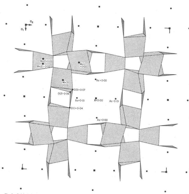
Fig. 2a. Polyhedral representation of the magnussonite crystal structure, z = 0. The basal oxygens associated with (AsO<sub>3</sub>) form a shaded triangle. The site "X" corresponds to MX(= Mn<sup>1+</sup>) centrally located and octahedrally coordinated by six As atoms, four of which occur in the section of the structure. Heights are given as fractional coordinates in z.
