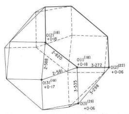
Fig. 4. The oxygen polyhedron, consisting of eighteen vertices, which is centered on MX at  $1/2 \ 1/2 \ 0$ . It possesses point symmetry  $\overline{3}$ . The asymmetric unit of vertices and edge lengths are labelled.
