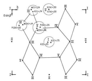
Fig. 3. The cations in the wyllieite structure (Moore and Molin-Case, 1974) with a portion of the  $\{6 \cdot 3 \cdot 6 \cdot 3\}$  and  $\{6 \cdot 6 \cdot 3 \cdot 3\}$  net drawn in. The structure is projected down [001] and preserves the axes and coordinates of the original study.
