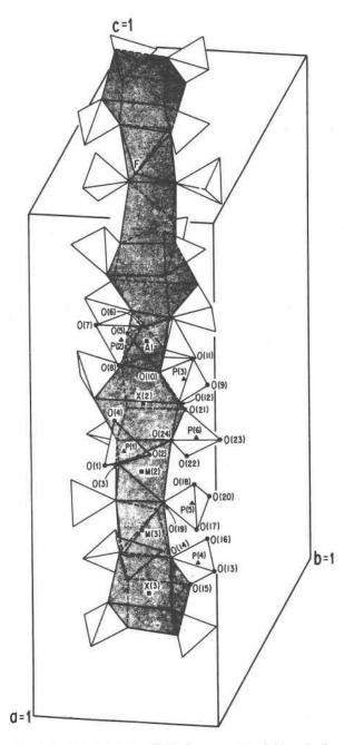
Fig. 4. Rod I in arrojadite (NM) drawn as a Penfield projection (Moore, 1981). The larger polyhedra are stippled and the enveloping transparent (PO<sub>4</sub>) tetrahedra are drawn in. Note the sequence cube-octahedron-square pyramid-cube-octahedron-square pyramid-octahedron-cube. The Al site is an inversion center.
