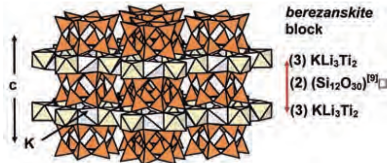
FIG. 4. General view of the crystal structure of berzanskite [drawn using atom coordinates of the sogdianite end-member, K^{[9]} \square Li_3 Zr_2 (Si_{12}O_{30}) , from Sokolova et al. (2000)]. Sheets (2) and (3) as in faizievite are shown within the berzanskite block (a red double-headed arrow). Legend as in Figure 1.
